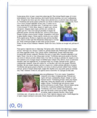
The PDF format is without resolution. This means that pages should be displayable at any zoom with consistent fidelity. Pages, however do have measurements. Pages are measured in default user space units, which are 1/72 inch. Although it is possible for a PDF file to specify other units for page measurement, it is rare.
