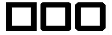
Paths may be stroked in an arbitrary dash pattern. The pattern is a phase number and a collection of alternating dash lengths and gap lengths. The dash and gap lengths are distances along the path in PDF units. The phase is how far into the pattern to start a line. The entire collection of dash and gaps is used until it is exhausted, then it is repeated until the complete path has been stroked.
