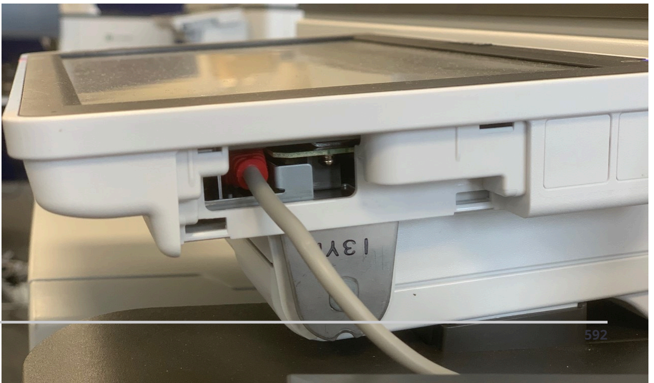
Card reader cable connected on Ricoh IM C3000
