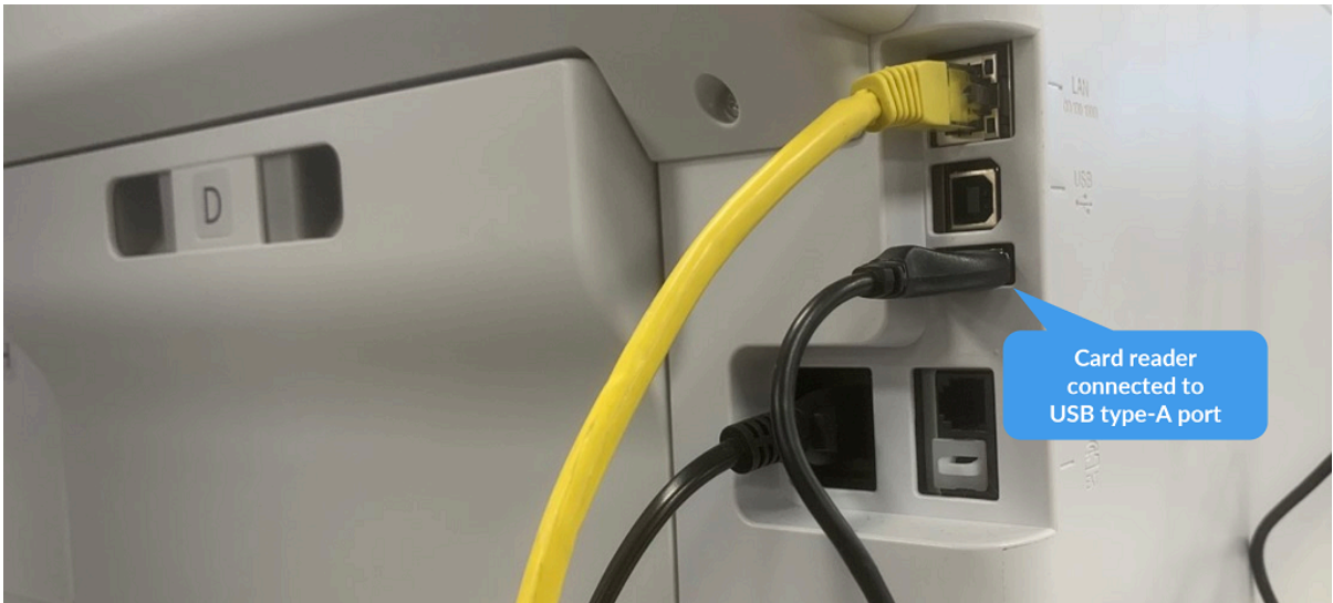
Card reader cable connected on Epson WF-C5790
