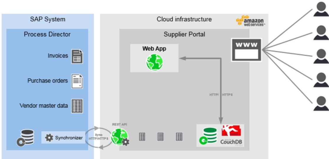
The synchronization is always initiated from Synchronizer in the SAP systems. All connections are outbound. No port needs to be open for an inbound connection to the SAP systems. The synchronization can be configured to use either SSL or plain HTTP. For security reasons, it is recommended to use SSL.
